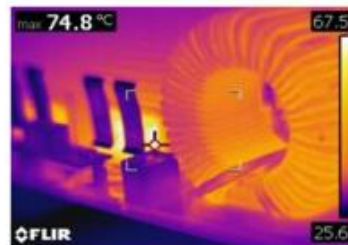
Figure 19. MOSFET Case Temperature (Q1)
