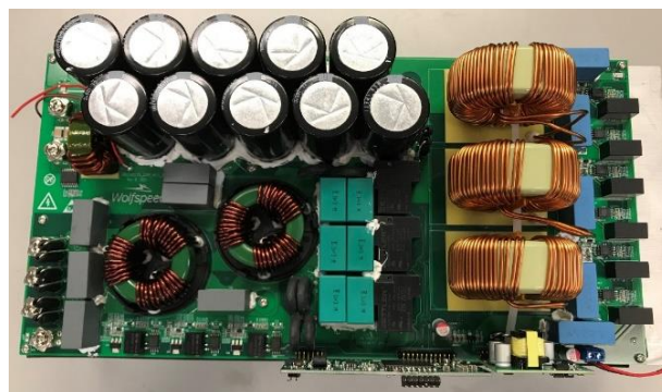
Figure 6. Wolfspeed 22kW Bi-Directional Charger Reference Design CRD-22AD12N
