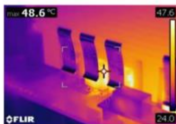
Figure 20. Diode Case Temperature (D25)
