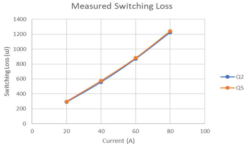
**Figure 6:** Measured switching losses of Q2 and Q5 at various currents
