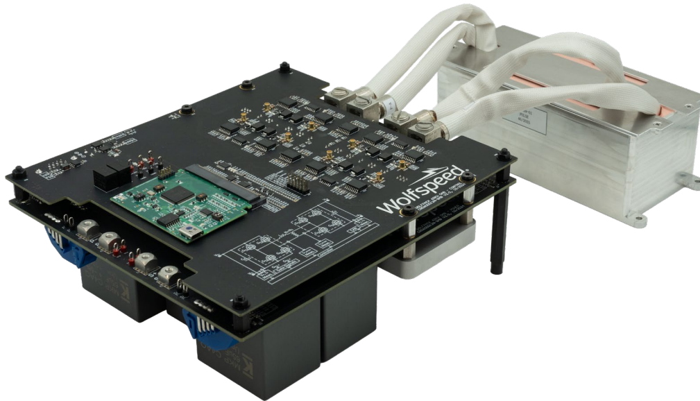
Figure 54: CRD60DD12N-GMB connected to YAGEO transformer
