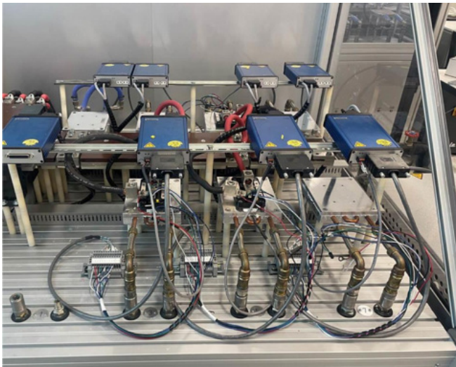
Figure 7: Up to 12 half-bridges power modules can be tested simultaneously
