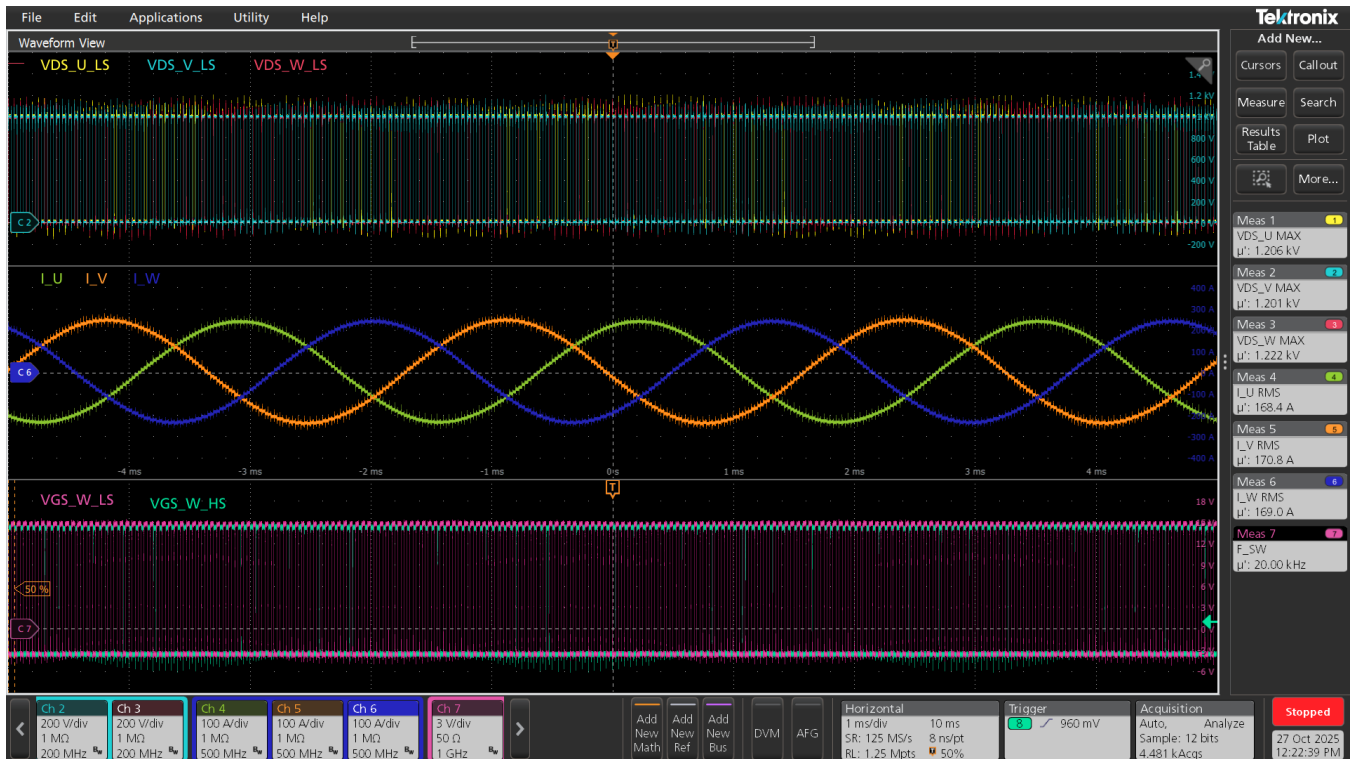
Figure 49: Oscilloscope measurements at 1 kV and 167 A
