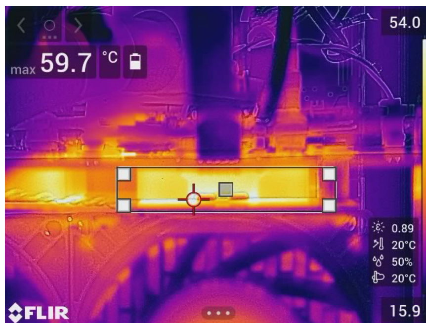
Figure 51: Phase W module temperature at 1 kV and 167 A
