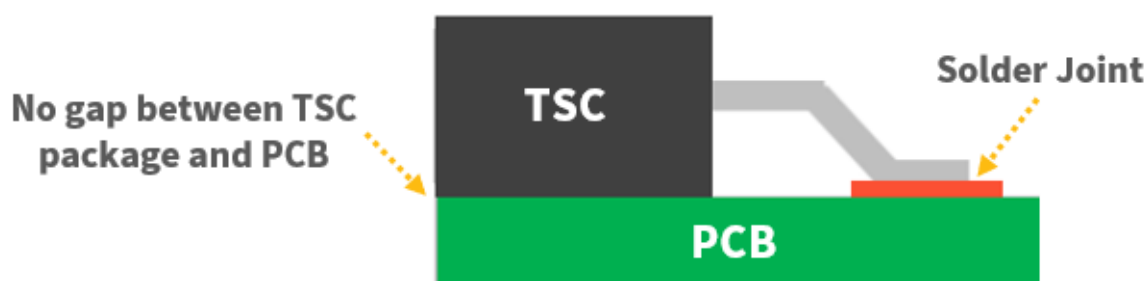
Figure 8: Example of Negative Standoff Design
