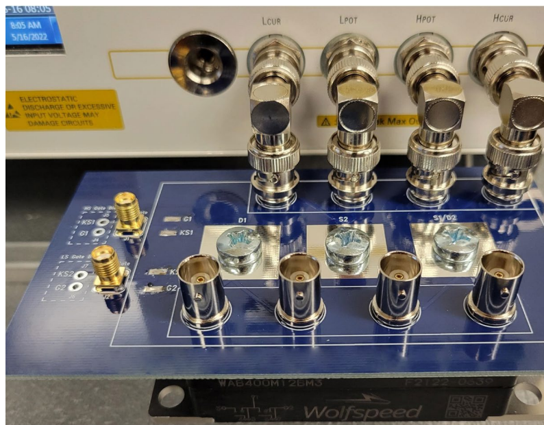
Figure 14: Example custom fixture for measuring a 62 mm power module [6]
