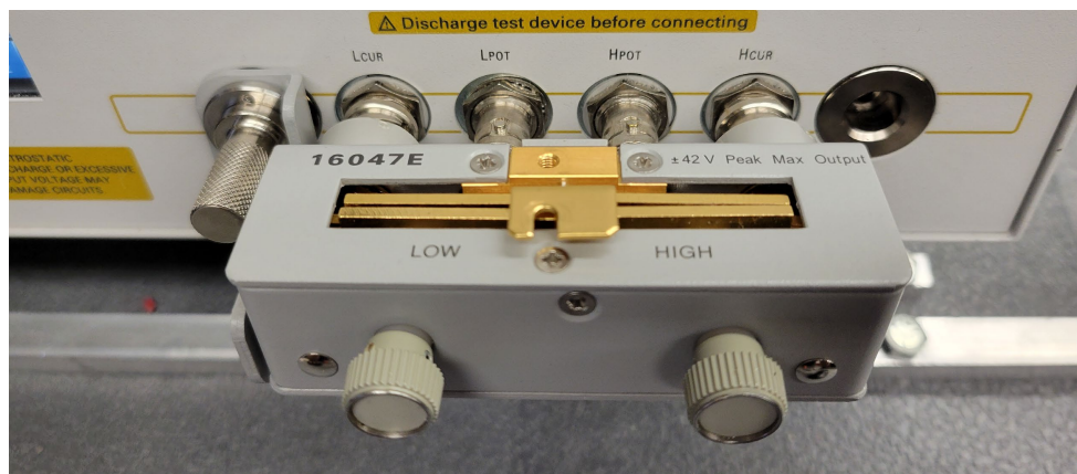
Figure 17: 16047e fixture attached to the E4990a impedance analyzer with the shorting bar attached
