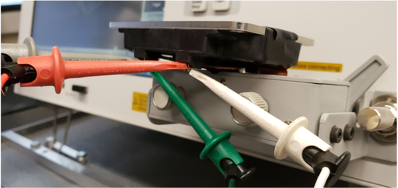
Figure 24: XM module measurement with 16047e fixture
