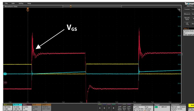
Figure 55: Distorted V_{GS} Waveform
