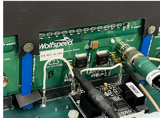
Figure 50: Oscilloscope probe connections
