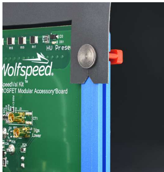
Figure 21: Fan shroud keyhole slot attachment
