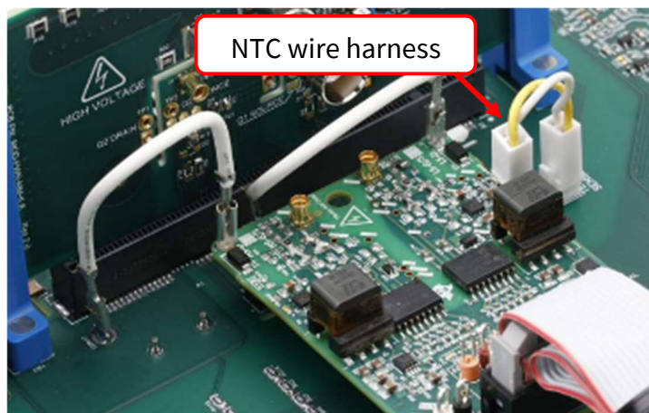
Figure 17: NTC sensing connection between motherboard and gate driver
