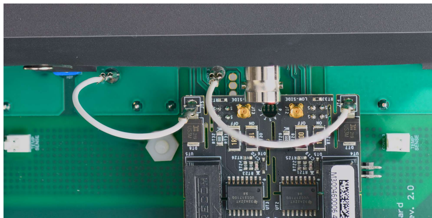
Figure 12: Drain Voltage Sense Jumpers
