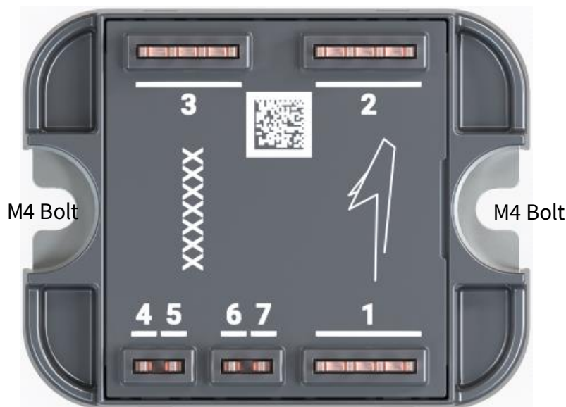
Figure 3: DM3 Mounting Bolt Pattern
