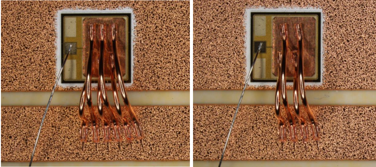
Figure 10: Wolfspeed die with DTS® Open Tool and 400 \mu\text{m} PowerCu Soft: Left image: 4-wire layout. Right image: 6-wire layout.
