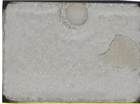
Figure 4: DTS backside showing a “paste chipping” after picking.
