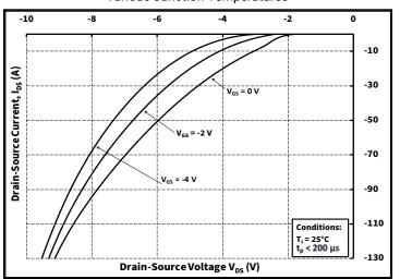
Figure 9. Body Diode Characteristic at 25 °C
