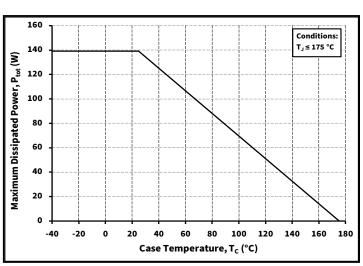
Figure 20. Maximum Power Dissipation Derating vs. Case Temperature
