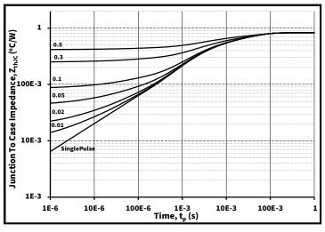
Figure 21. Transient Thermal Impedance (Junction - Case)
