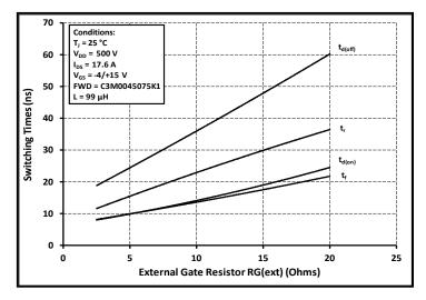
Figure 27. Switching Times vs. R<sub>G(ext)</sub>
