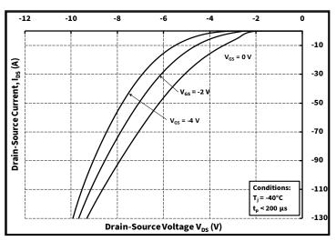
Figure 8. Body Diode Characteristic at -40 °C
