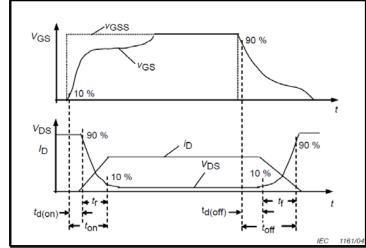
Figure 28. Switching Times Definition
