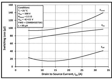
Figure 24. Clamped Inductive Switching Energy vs. Drain Current (V<sub>DD</sub> = 500V)
