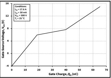
Figure 12. Gate Charge Characteristics
