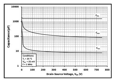
Figure 18. Capacitances vs. Drain-Source Voltage (0 - 750V)
