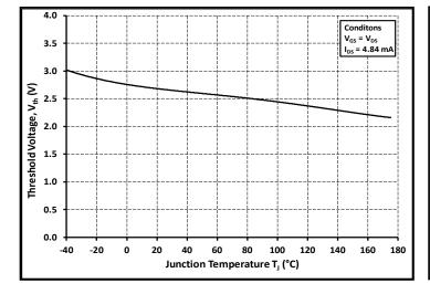
Figure 11. Threshold Voltage vs. Temperature
