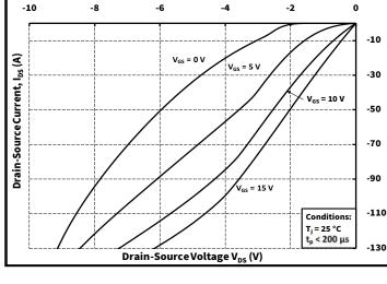
Figure 14. 3rd Quadrant Characteristic at 25 °C
