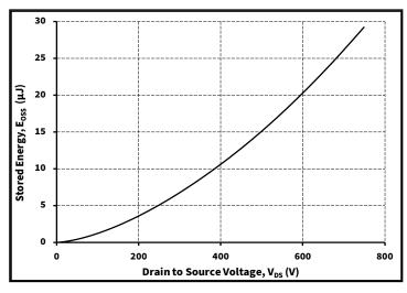
Figure 16. Output Capacitor Stored Energy
