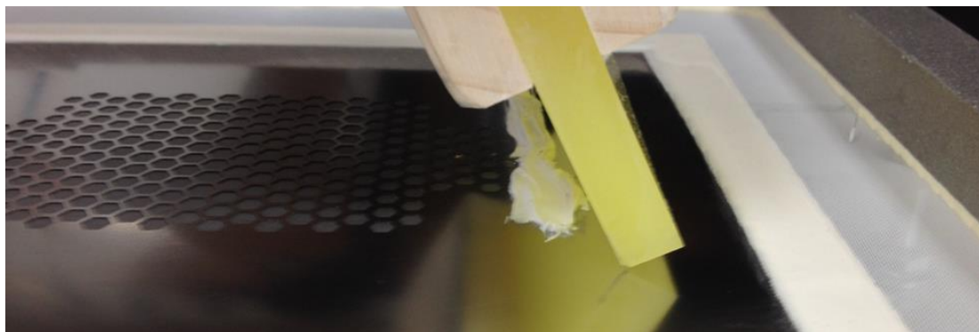
Figure 13. Suggested squeegee application angle
