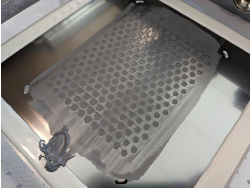
Figure 14. Correct application of TIM to stencil
