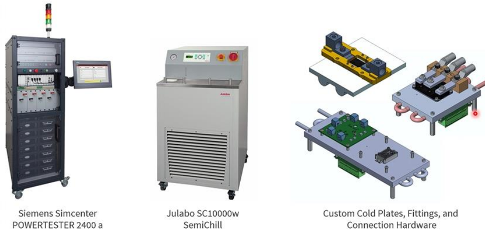
Figure 19: Thermal transient test equipment
