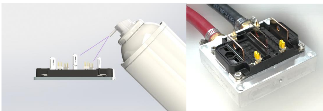
Figure 21: Emissivity coating application method
