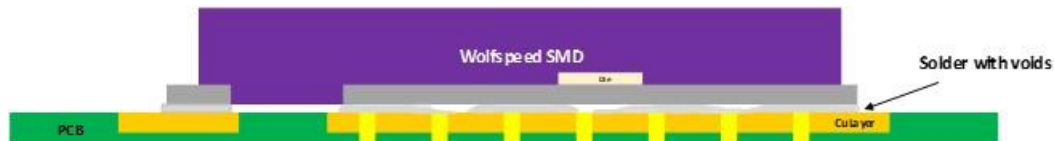
Figure 10: Solder Joint with Voids for SMDs
