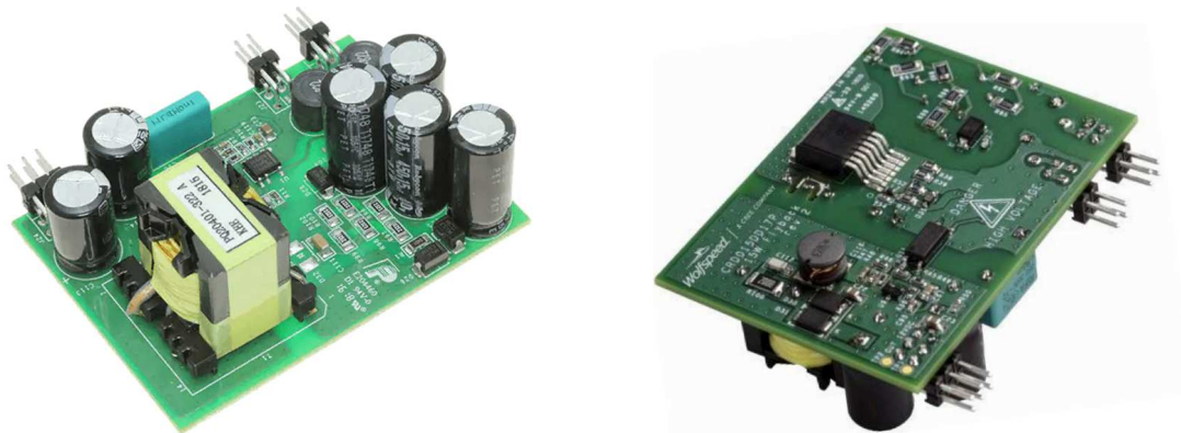
Figure 1: Wolfspeed's CRD15DD17P, 15 W flyback auxiliary power supply board
