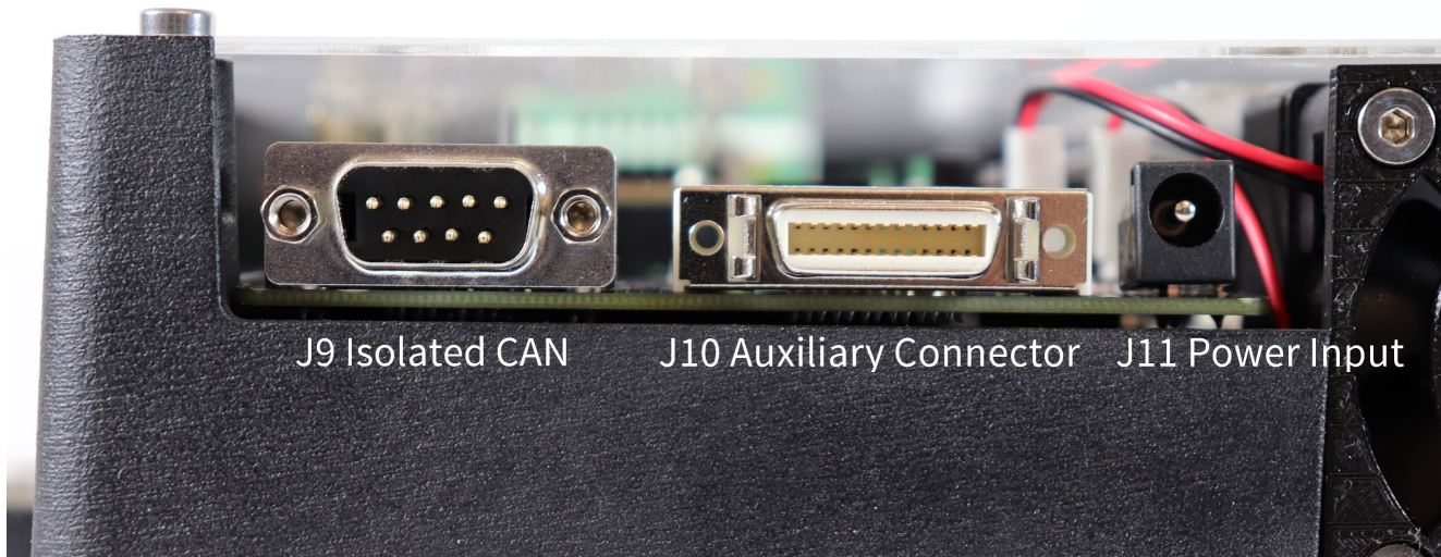
Figure 6. Left Side View Showing Controller Interfaces Connectors
