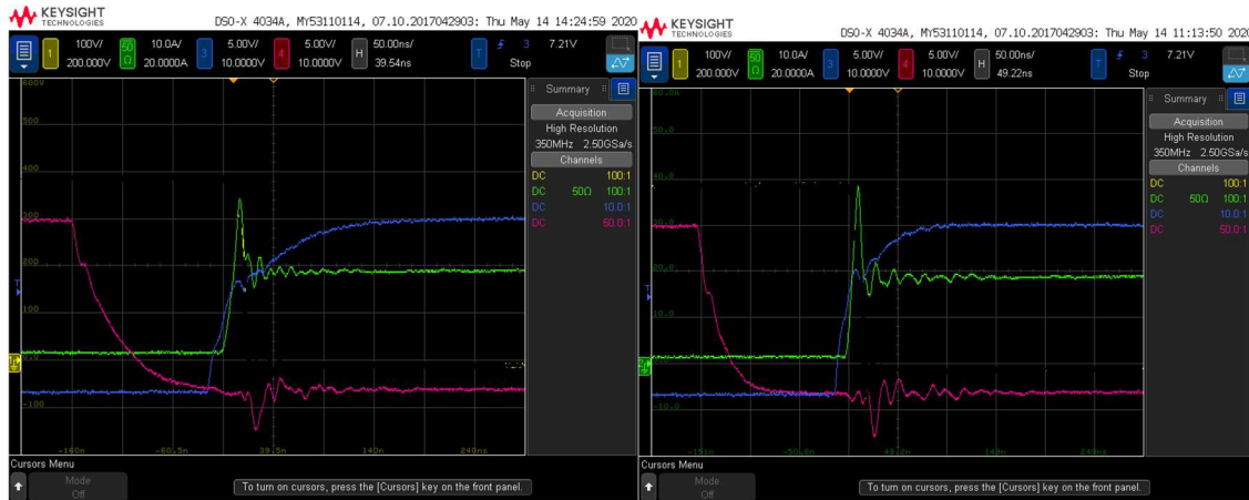
Figure 8: Turn-on switching transition at 3.5kW for R_g=12 (left) and R_g=6 (right). Note that the negative voltage seen on the Q2 V_{gs} is a measurement artifact
