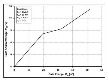
Figure 12. Gate Charge Characteristics
