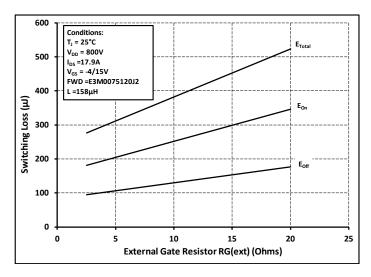
Figure 25. Clamped Inductive Switching Energy vs.  $R_{G(ext)}$
