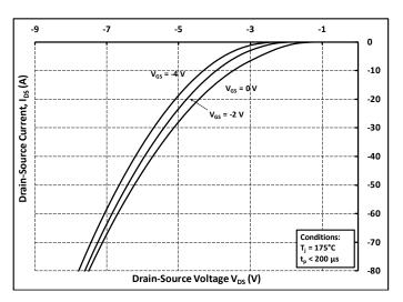
Figure 10. Body Diode Characteristic at 175 °C
