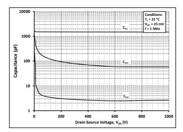
Figure 18. Capacitances vs. Drain-Source Voltage (0 - 1200V)
