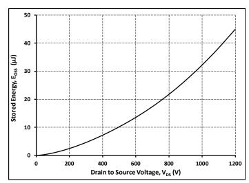
Figure 16. Output Capacitor Stored Energy
