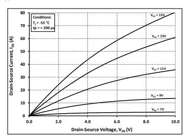
Figure 1. Output Characteristics T<sub>J</sub> = -55 °C
