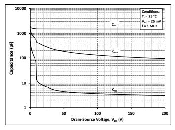
Figure 17. Capacitances vs. Drain-Source Voltage (0 - 200V)
