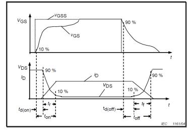
Figure 28. Switching Times Definition
