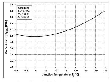
Figure 4. Normalized On-Resistance vs. Temperature
