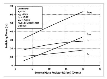
Figure 27. Switching Times vs.  $R_{G(ext)}$
