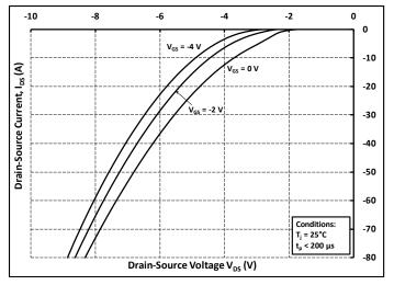
Figure 9. Body Diode Characteristic at 25 °C
