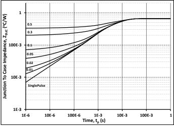
Figure 21. Transient Thermal Impedance (Junction - Case)
