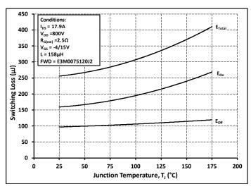
Figure 26. Clamped Inductive Switching Energy vs.
