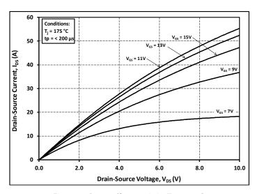
Figure 3. Output Characteristics T<sub>J</sub> = 175 °C
