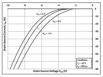
Figure 8. Body Diode Characteristic at -55 °C
