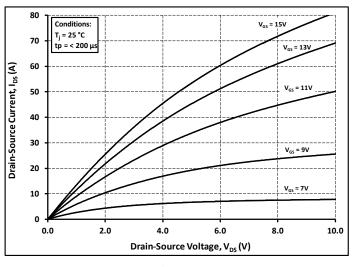
Figure 2. Output Characteristics T<sub>J</sub> = 25 °C
