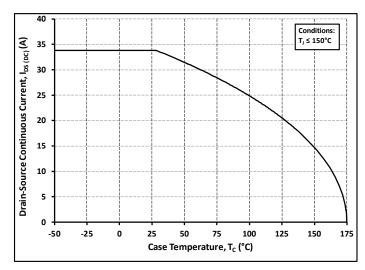
Figure 19. Continuous Drain Current Derating vs.
