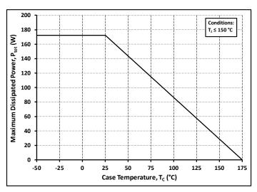
Figure 20. Maximum Power Dissipation Derating vs.
