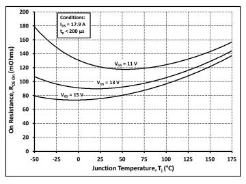
Figure 6. On-Resistance vs. Temperature For Various Gate Voltage
