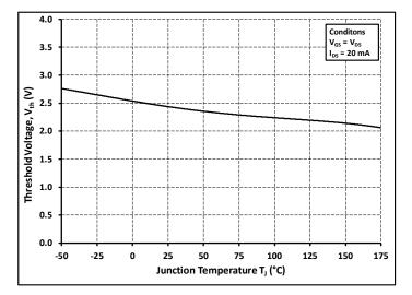
Figure 11. Threshold Voltage vs. Temperature
