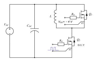
Figure 29. Clamped Inductive Switching Waveform Test Circuit
