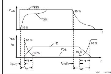
Figure 28. Switching Times Definition
