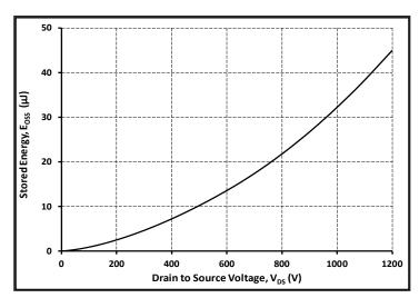
Figure 16. Output Capacitor Stored Energy
