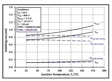
Figure 26. Clamped Inductive Switching Energy vs.
