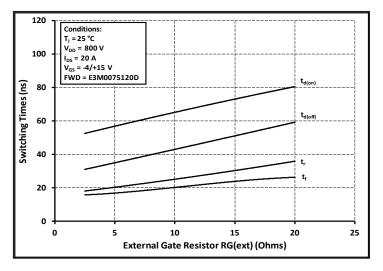
Figure 27. Switching Times vs.  $R_{G(ext)}$
