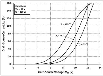
Figure 7. Transfer Characteristic for Various Junction Temperatures
