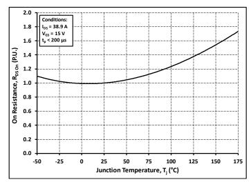
Figure 4. Normalized On-Resistance vs. Temperature
