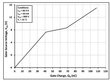
Figure 12. Gate Charge Characteristics
