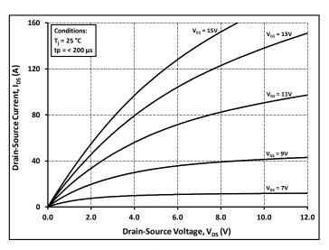
Figure 2. Output Characteristics T<sub>J</sub> = 25 °C
