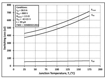
Figure 26. Clamped Inductive Switching Energy vs.
