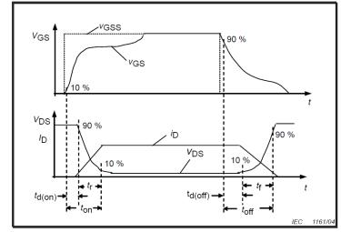
Figure 28. Switching Times Definition
