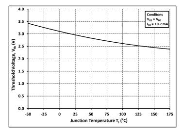
Figure 11. Threshold Voltage vs. Temperature
