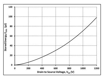
Figure 16. Output Capacitor Stored Energy
