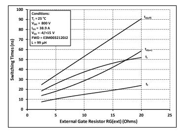
Figure 27. Switching Times vs.  $R_{G(ext)}$
