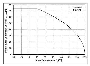
Figure 19. Continuous Drain Current Derating vs.
