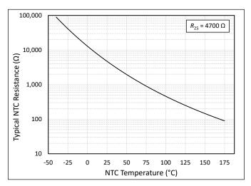
Figure 6. NTC Resistance vs. NTC Temperature
