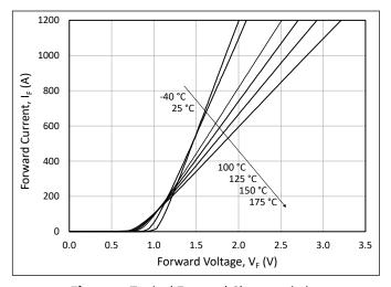
Figure 1. Typical Forward Characteristics
