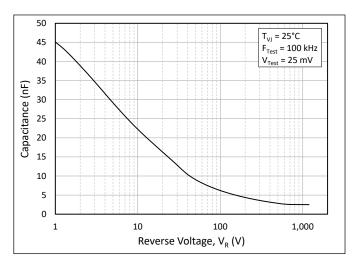
Figure 3. Typical Capacitance vs. Reverse Voltage
