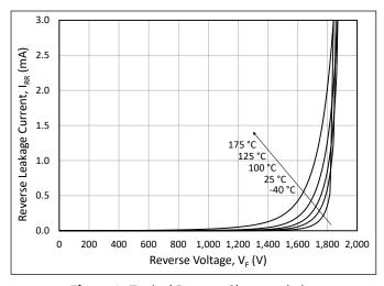
Figure 2. Typical Reverse Characteristics
