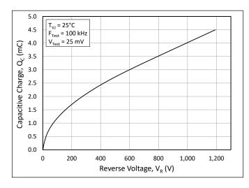
Figure 4. Typical Capacitive Charge vs. Reverse Voltage
