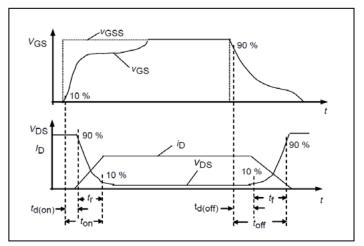
Figure 28. Switching Times Definition
