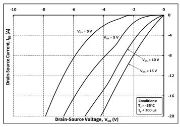
Figure 13. 3rd Quadrant Characteristic at -55°C
