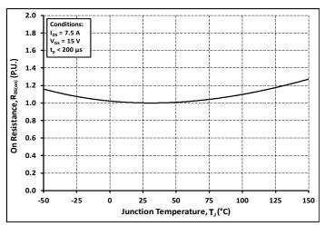
Figure 4. Normalized On-Resistance vs Temperature
