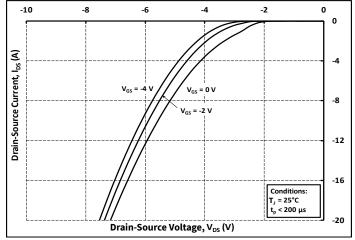
Figure 9. Body Diode Characteristic at 25°C
