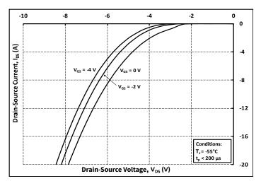
Figure 8. Body Diode Characteristic at -55°C
