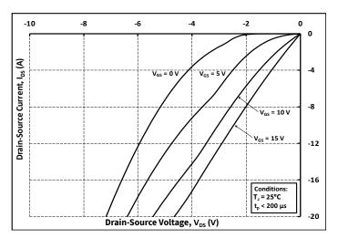
Figure 14. 3rd Quadrant Characteristic at 25°C
