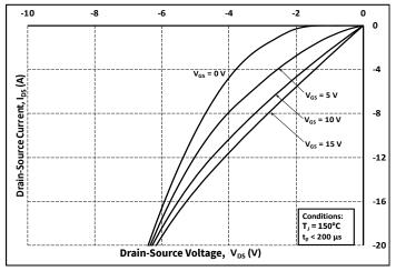
Figure 15. 3rd Quadrant Characteristic at 150°C
