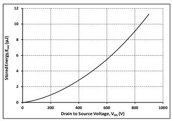
Figure 16. Output Capacitor Stored Energy
