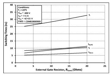
Figure 27. Switching Times vs. R<sub>G(ext)</sub>
