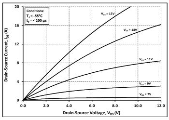
Figure 1. Output Characteristics T<sub>J</sub> = -55°C
