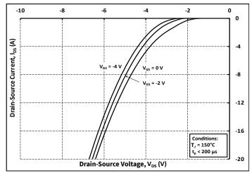
Figure 10. Body Diode Characteristic at 150°C
