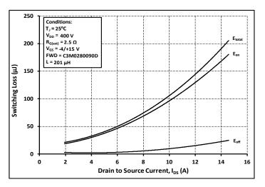
**Figure 24.** Clamped Inductive Switching Energy vs Drain Current (V<sub>DD</sub> = 400 V)
