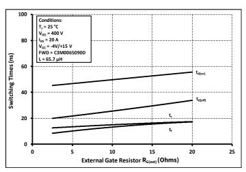
Figure 27. Switching Times vs. R<sub>G(ext)</sub>
