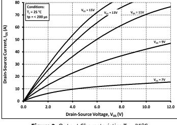
Figure 2. Output Characteristics T<sub>J</sub> = 25°C
