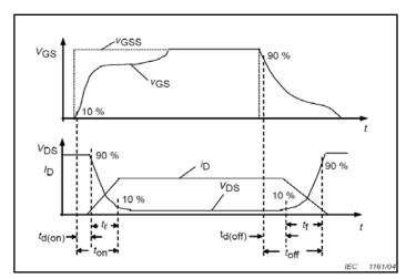
Figure 28. Switching Times Definition
