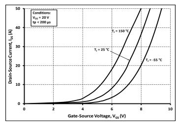
**Figure 7.** Transfer Characteristic for Various Junction Temperatures
