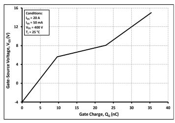
Figure 12. Gate Charge Characteristics
