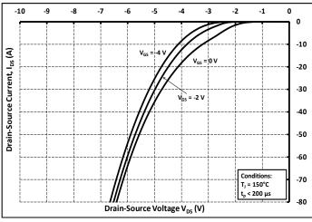
**Figure 10.** Body Diode Characteristic at 150°C
