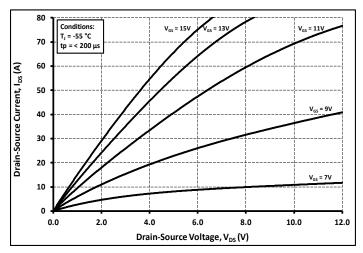
**Figure 1.** Output Characteristics  $T_J = -55^{\circ}C$
