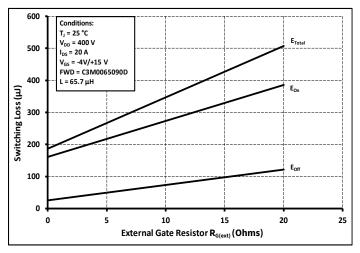
Figure 25. Clamped Inductive Switching Energy vs R<sub>G(ext)</sub>
