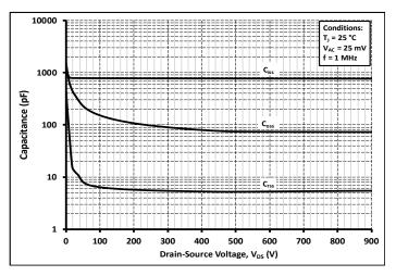
**Figure 18.** Capacitances vs Drain-Source Voltage (0 - 900 V)
