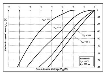
Figure 13. 3rd Quadrant Characteristic at -55°C
