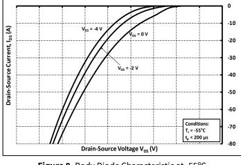
Figure 8. Body Diode Characteristic at -55°C
