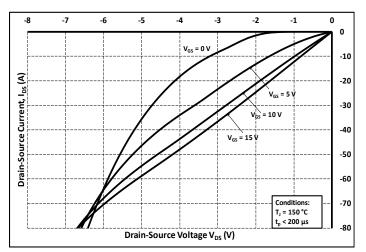
Figure 15. 3rd Quadrant Characteristic at 150°C
