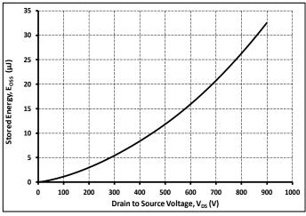
Figure 16. Output Capacitor Stored Energy
