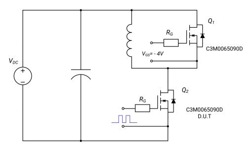
**Figure 30.** Clamped Inductive Switching Waveform Test Circuit
