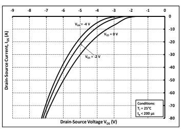
Figure 9. Body Diode Characteristic at 25°C
