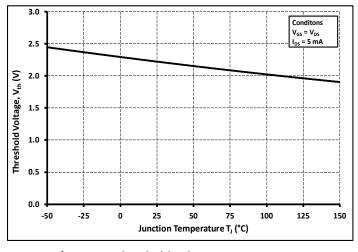
Figure 11. Threshold Voltage vs. Temperature
