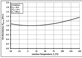
Figure 4. Normalized On-Resistance vs. Temperature
