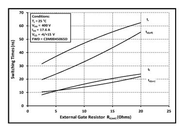
Figure 26. Switching Times vs. R<sub>G(ext)</sub>
