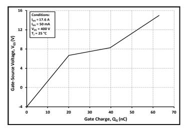
Figure 12. Gate Charge Characteristics
