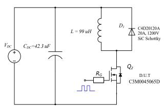
Figure 27. Clamped Inductive Switching Waveform Test Circuit
