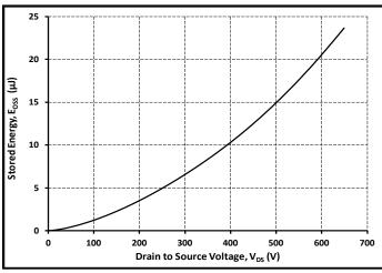
Figure 16. Output Capacitor Stored Energy
