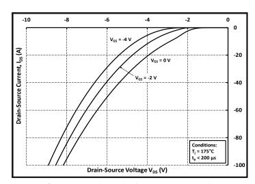
Figure 10. Body Diode Characteristic at 175°C
