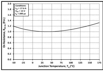
Figure 4. Normalized On-Resistance vs. Temperature
