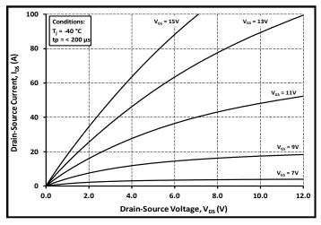
Figure 1. Output Characteristics T<sub>J</sub> = -40°C
