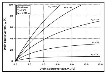
Figure 2. Output Characteristics T<sub>J</sub> = 25°C
