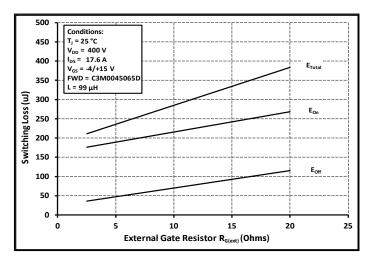
Figure 24. Clamped Inductive Switching Energy vs. R<sub>G(ext)</sub>
