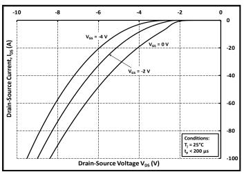
Figure 9. Body Diode Characteristic at 25°C
