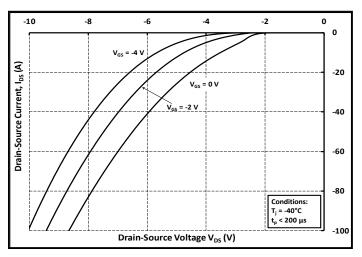
Figure 8. Body Diode Characteristic at -40°C
