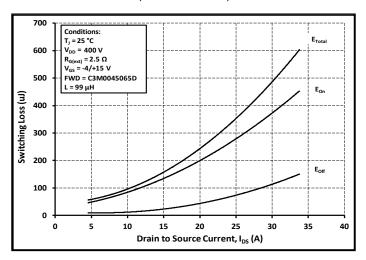
**Figure 23.** Clamped Inductive Switching Energy vs. Drain Current (V<sub>DD</sub> = 400 V)
