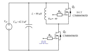
Figure 28. Body Diode Recovery Test Circuit
