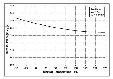
Figure 11. Threshold Voltage vs. Temperature
