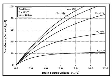
Figure 3. Output Characteristics T<sub>J</sub> = 175°C
