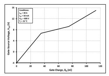
Figure 12. Gate Charge Characteristics
