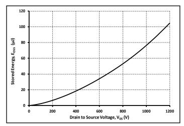
Figure 16. Output Capacitor Stored Energy
