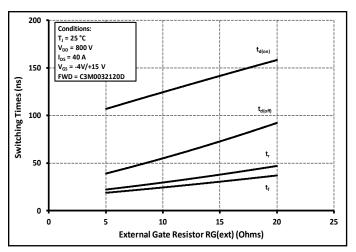
Figure 27. Switching Times vs. R<sub>G(ext)</sub>
