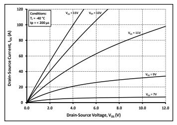
**Figure 1.** Output Characteristics  $T_J = -40^{\circ}C$
