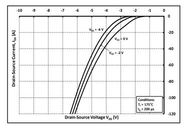
Figure 10. Body Diode Characteristic at 175°C
