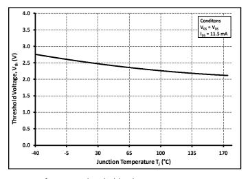
Figure 11. Threshold Voltage vs. Temperature
