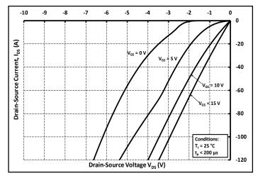
Figure 14. 3rd Quadrant Characteristic at 25°C
