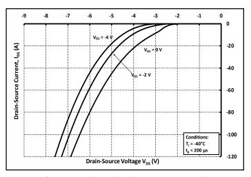
Figure 8. Body Diode Characteristic at -40°C
