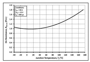
Figure 4. Normalized On-Resistance vs. Temperature
