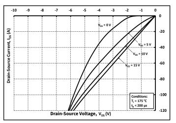
Figure 15. 3rd Quadrant Characteristic at 175°C
