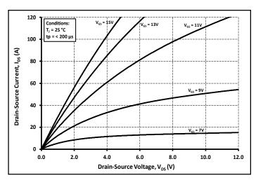
Figure 2. Output Characteristics  $T_1 = 25^{\circ}C$
