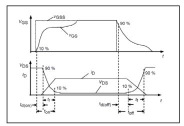
Figure 28. Switching Times Definition
