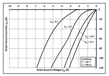
Figure 13. 3rd Quadrant Characteristic at -40°C
