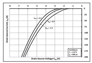
Figure 10. Body Diode Characteristic at 175°C
