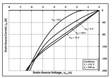
Figure 15. 3rd Quadrant Characteristic at 175°C
