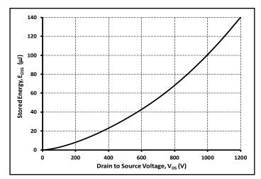
**Figure 16.** Output Capacitor Stored Energy
