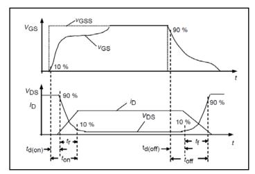
Figure 28. Switching Times Definition
