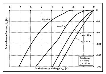
Figure 13. 3rd Quadrant Characteristic at -40°C
