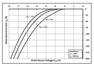
Figure 8. Body Diode Characteristic at -40°C
