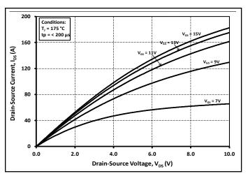
**Figure 3.** Output Characteristics  $T_J = 175$ °C
