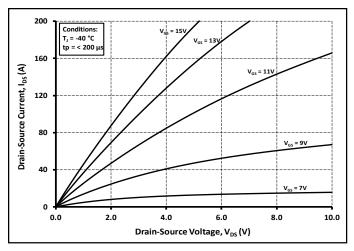
**Figure 1.** Output Characteristics  $T_J = -40^{\circ}C$
