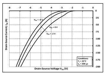
Figure 9. Body Diode Characteristic at 25°C
