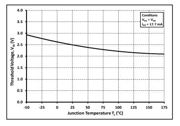
Figure 11. Threshold Voltage vs. Temperature
