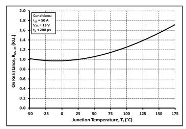
Figure 4. Normalized On-Resistance vs. Temperature
