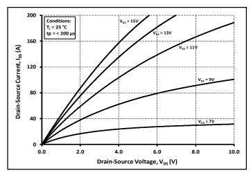
Figure 2. Output Characteristics  $T_1 = 25^{\circ}C$
