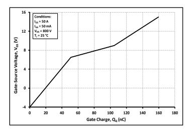
Figure 12. Gate Charge Characteristics
