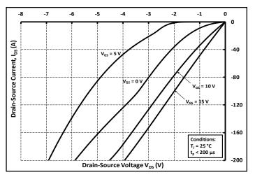
Figure 14. 3rd Quadrant Characteristic at 25°C
