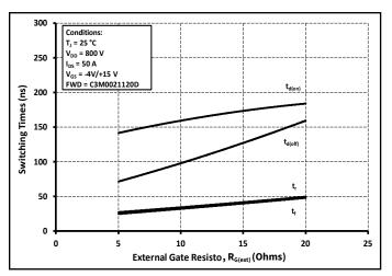
Figure 27. Switching Times vs. R<sub>G(ext)</sub>
