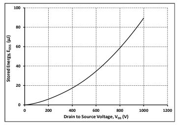
Figure 16. Output Capacitor Stored Energy
