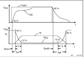
Figure 28. Switching Times Definition
