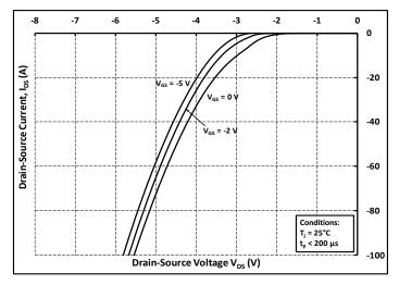
Figure 9. Body Diode Characteristic at 25°C
