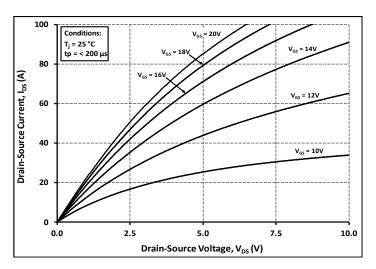
Figure 2. Output Characteristics T<sub>J</sub> = 25°C
