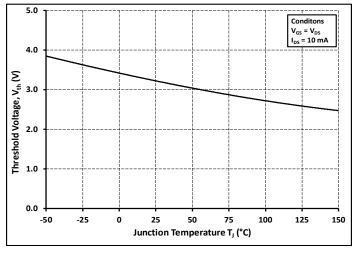
Figure 11. Threshold Voltage vs. Temperature
