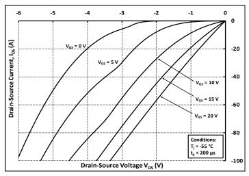
Figure 13. 3rd Quadrant Characteristic at -55°C
