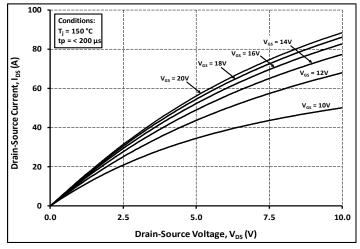
Figure 3. Output Characteristics T<sub>J</sub> = 150°C
