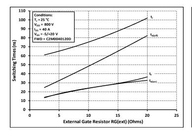
Figure 27. Switching Times vs. R<sub>G(ext)</sub>
