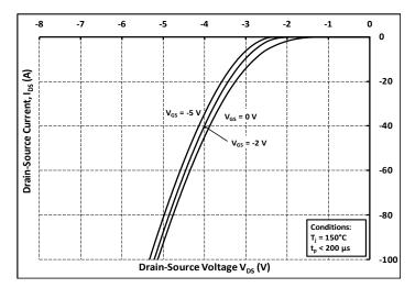
Figure 10. Body Diode Characteristic at 150°C
