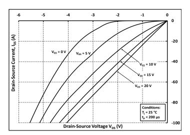
Figure 14. 3rd Quadrant Characteristic at 25°C
