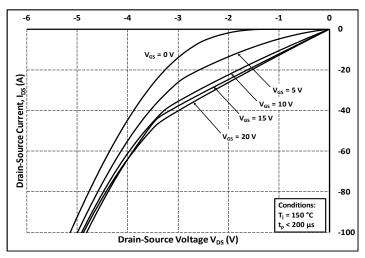
Figure 15. 3rd Quadrant Characteristic at 150°C
