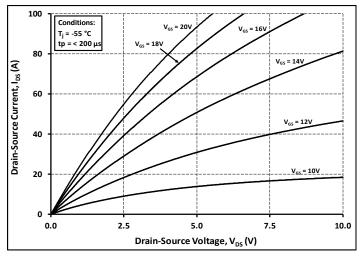
Figure 1. Output Characteristics T<sub>J</sub> = -55°C
