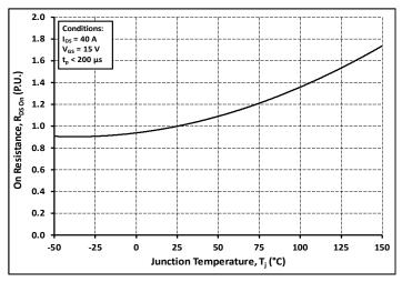
Figure 4. Normalized On-Resistance vs. Temperature
