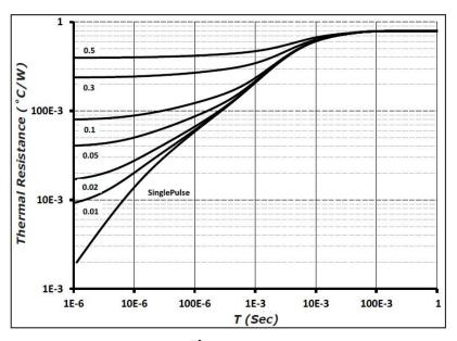
Figure 9 Transient Thermal Impedance
