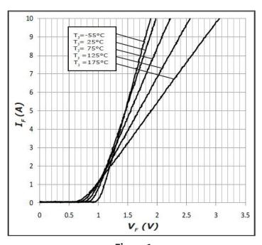
**Figure 1**Forward Characteristics
