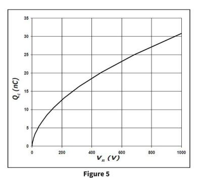
Total Capacitance Charge vs. Reverse Voltage
