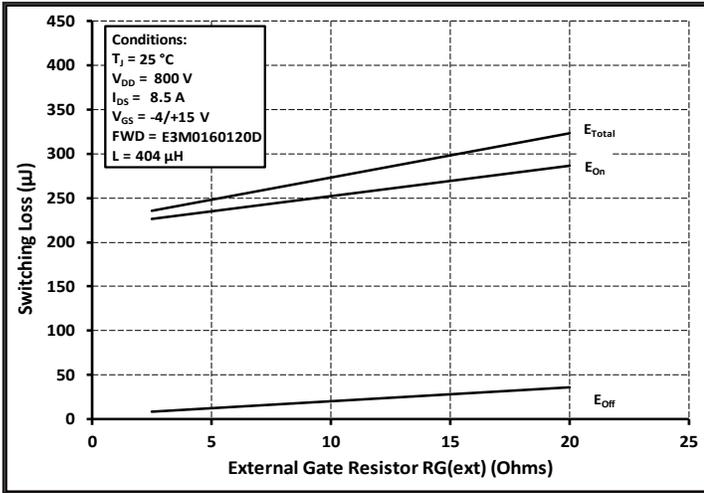
Figure 25. Clamped Inductive Switching Energy vs.  $R_{G(ext)}$
