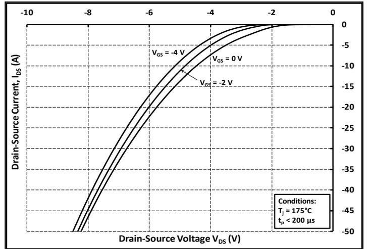
Figure 10. Body Diode Characteristic at 175 °C
