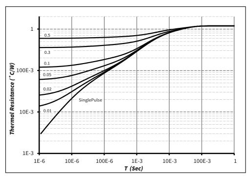
Figure 9. Transient Thermal Impedance
