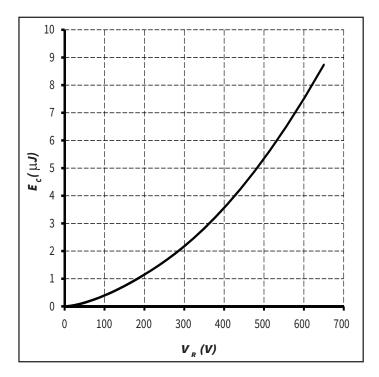
Figure 7. Capacitance Stored Energy
