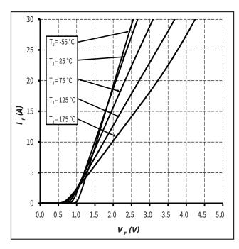
Figure 1. Forward Characteristics
