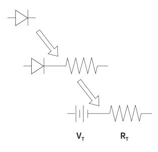
$Vf_{T} = V_{T} + If^{*}R_{T}$  $V_{T} = 0.94 + (T_{J}^{*} - 1.3^{*}10^{-3})$  $R_{T} = 0.044 + (T_{J}^{*} 4.4^{*}10^{-4})$
