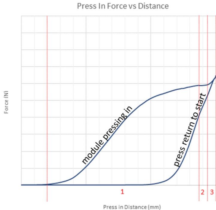
Figure 10. Typical press-in force profile for WolfPACK™ series module
