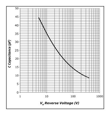
Figure 4. Capacitance vs. Reverse Voltage
