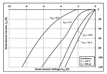
Figure 13. 3rd Quadrant Characteristic at -40°C
