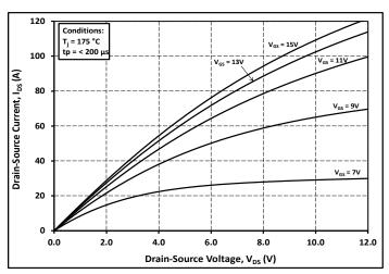
Figure 3. Output Characteristics T<sub>J</sub> = 175°C
