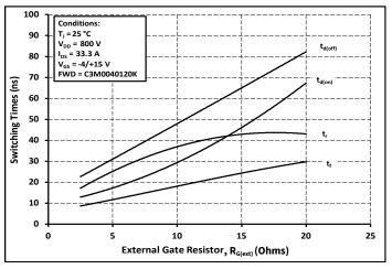
Figure 27. Switching Times vs. R<sub>G(ext)</sub>
