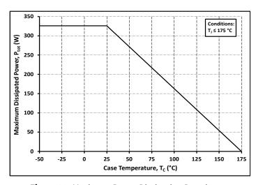
**Figure 20.** Maximum Power Dissipation Derating vs. Case Temperature
