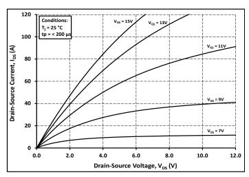
Figure 2. Output Characteristics T<sub>J</sub> = 25°C
