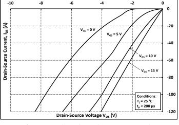
Figure 14. 3rd Quadrant Characteristic at 25°C
