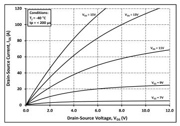
Figure 1. Output Characteristics T<sub>J</sub> = -40°C
