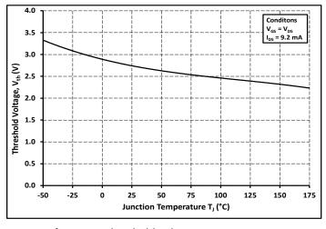
Figure 11. Threshold Voltage vs. Temperature
