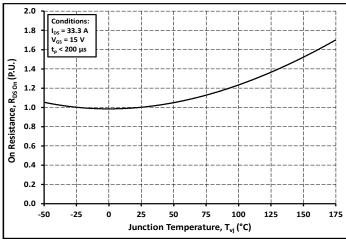
Figure 4. Normalized On-Resistance vs. Temperature
