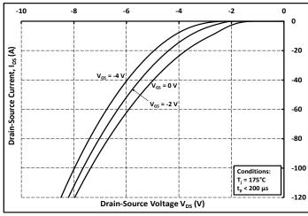
Figure 10. Body Diode Characteristic at 175°C
