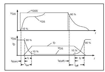
Figure 28. Switching Times Definition
