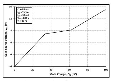
Figure 12. Gate Charge Characteristics
