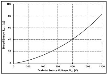
Figure 16. Output Capacitor Stored Energy
