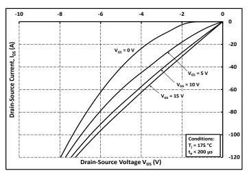
Figure 15. 3rd Quadrant Characteristic at 175°C
