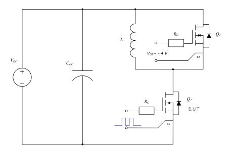
Figure 29. Clamped Inductive Switching Waveform Test Circuit
