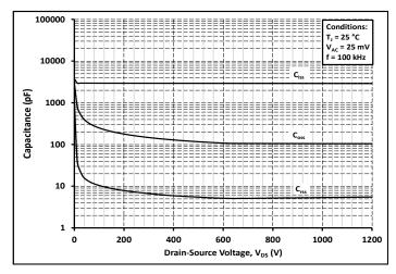
**Figure 18.** Capacitances vs. Drain-Source Voltage (0 - 1200 V)
