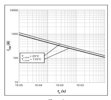
**Figure 8**Non Repetitive Peak Forward Surge Current versus Pulse Duration (sinsusoidal waveform)
