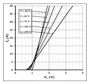
**Figure 1**Forward Characteristics
