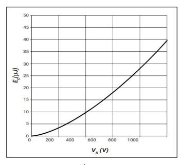
**Figure 7**Capacitance Stored Energy
