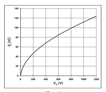
**Figure 5**Total Capacitance vs. Reverse Voltage
