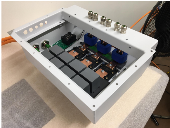
Fig. 2. An open view of the HV section of the inverter
