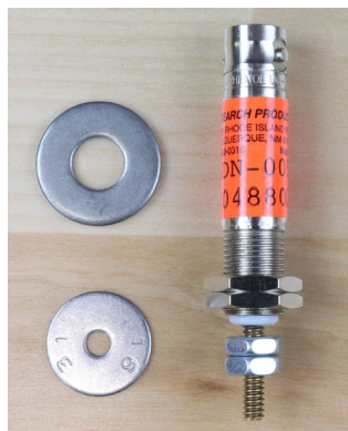
Figure 14: T&M Research ® SSDN tubular current shunt
