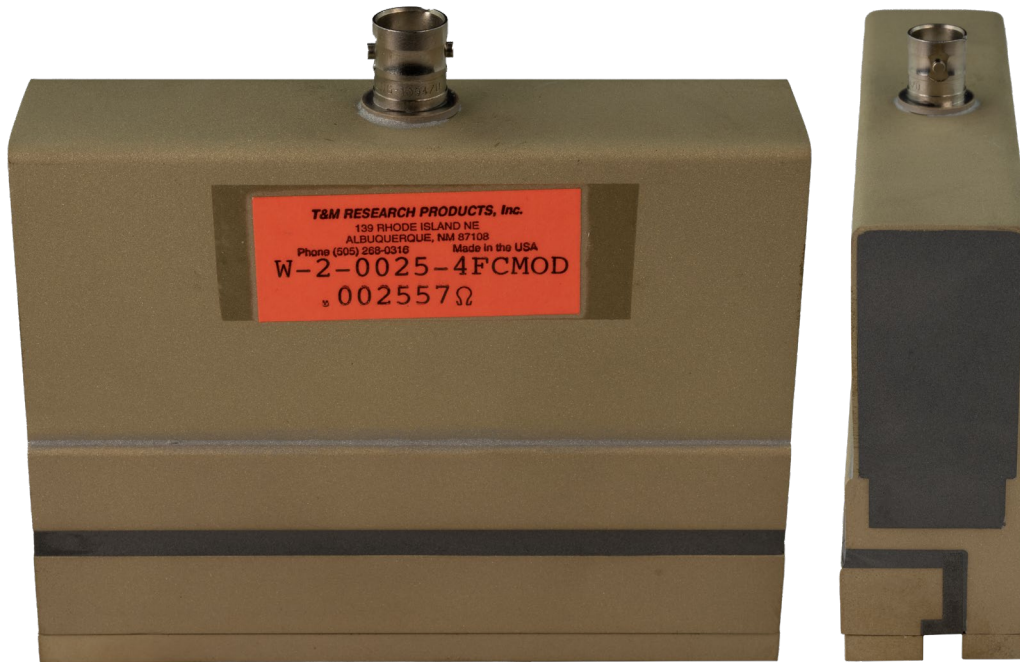
Figure 15: T&M Research® W-2-0025-4FC 2.5 mΩ CVR
