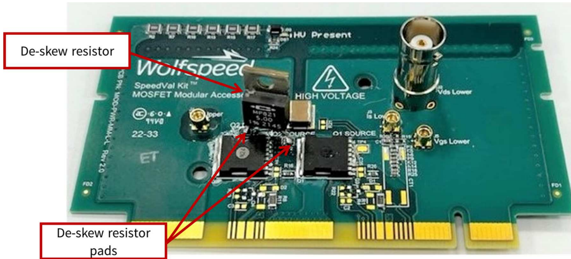
Figure 8: Deskew resistor position on the power TOLL power daughter card
