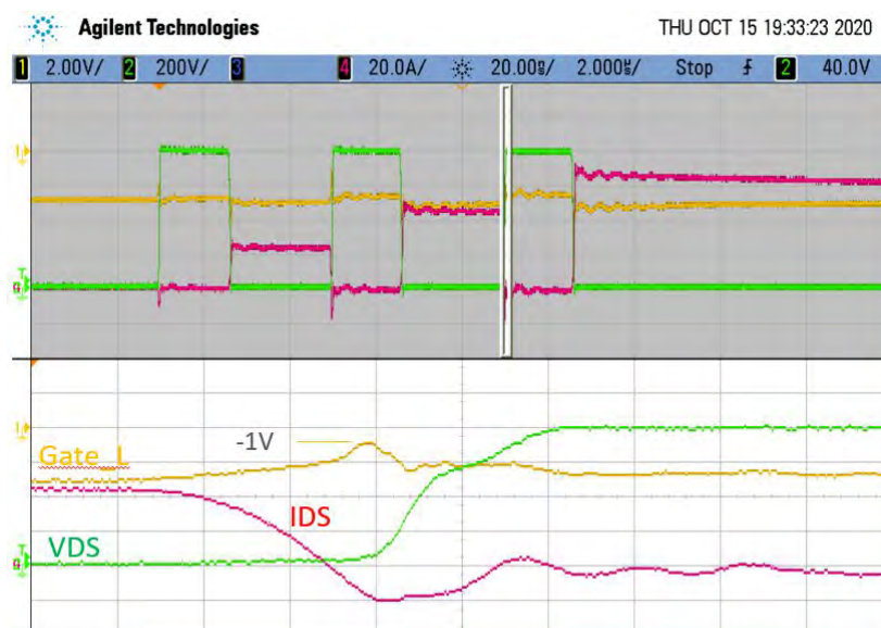
Figure 9: C3M0016120K with R_G=10\text{ohms} , V_{DS}=800\text{V}
