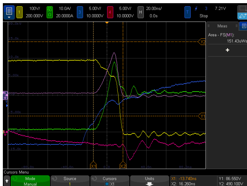
Figure 14: Example of turn-on waveforms
