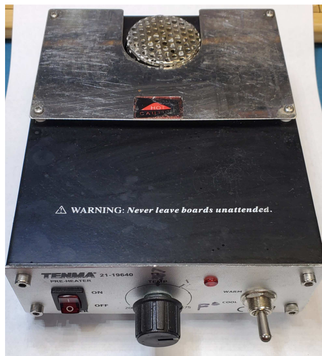
Figure 3: A benchtop PCB preheating tool
