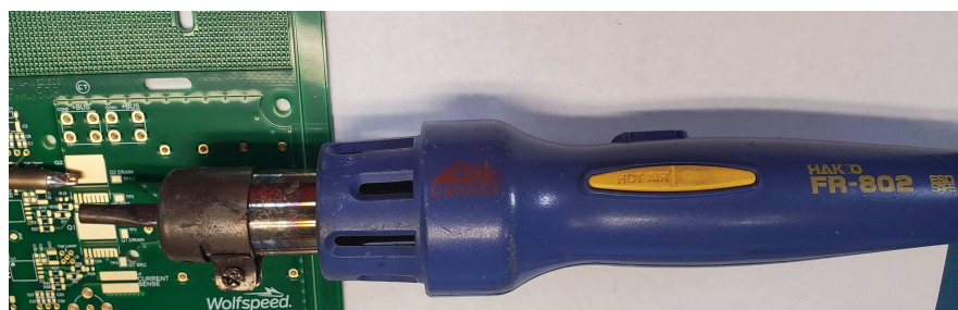
Figure 4: Hot-air pen for manual soldering or rework
