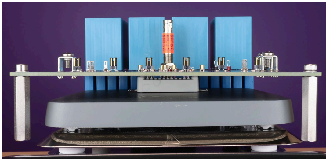
Figure 28: FM3 Module on Hot Plate for Elevated Temperature Testing
