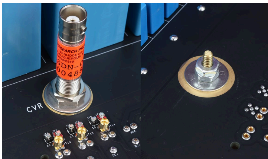
Figure 18: Tubular SSDN CVR Installed in PCB from Top View (Left) and Bottom View (Right)
