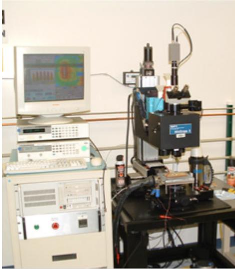
Figure 1 – Infrascopie II Set-up
