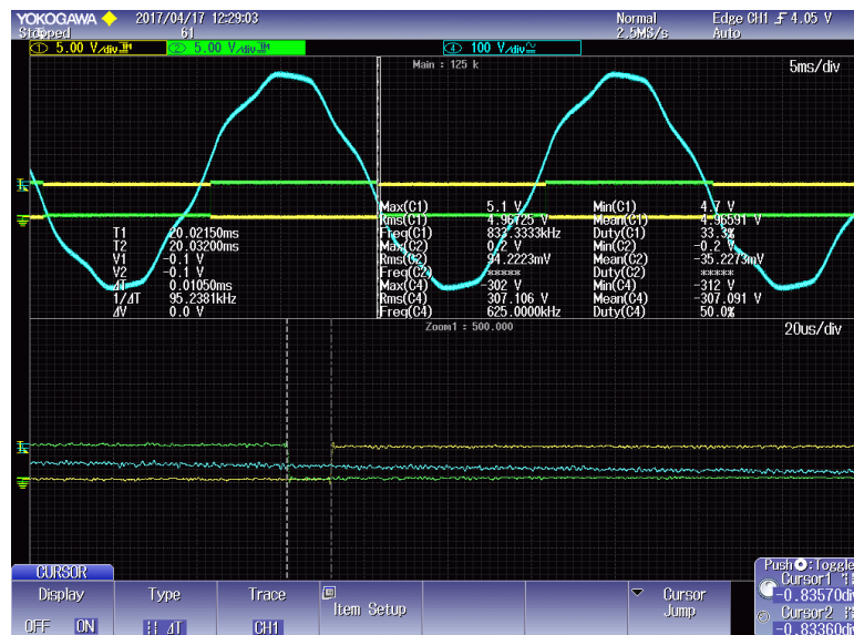
Figure 19: Input voltage ( V_{in} ) and dead band waveforms at V_{in} = 100 VAC
