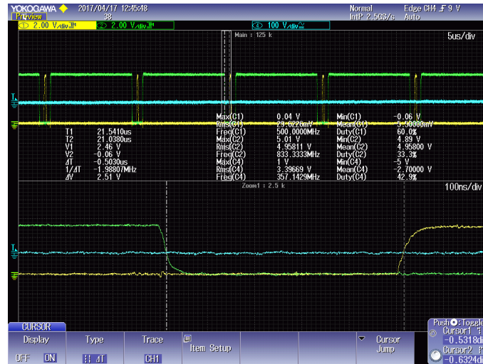
Figure 22: Deadtime between the top and the bottom PWM signals
