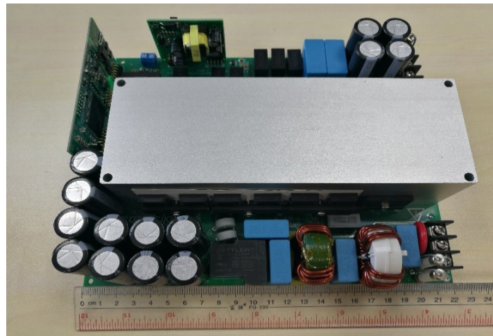
Figure 4: 6.6 kW bidirectional OBC prototype based on TO-247 650 V SiC MOSFET.
