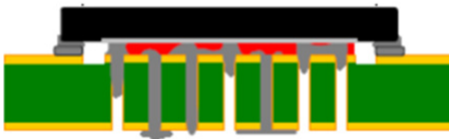
Figure 1: Solder voiding due to wicking of solder into copper-plated thermal via under the device
