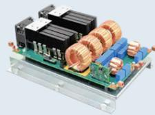
**60 kW INTERLEAVED BOOST CONVERTER**
