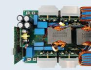
**22 kW Bi-Directional CLLC Utilizing IMS Board**
