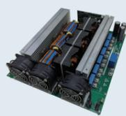
**30 kW DISCRETE INTERLEAVED LLC DC-DC CONVERTER**
