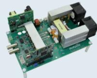
**6.6 kW High Frequency DC-DC Converter**
