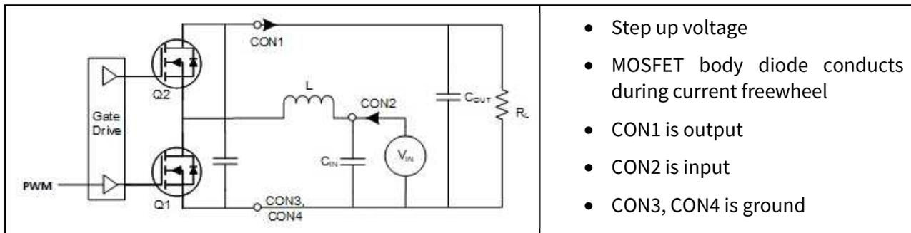
Figure 6: Asynchronous boost converter configuration
