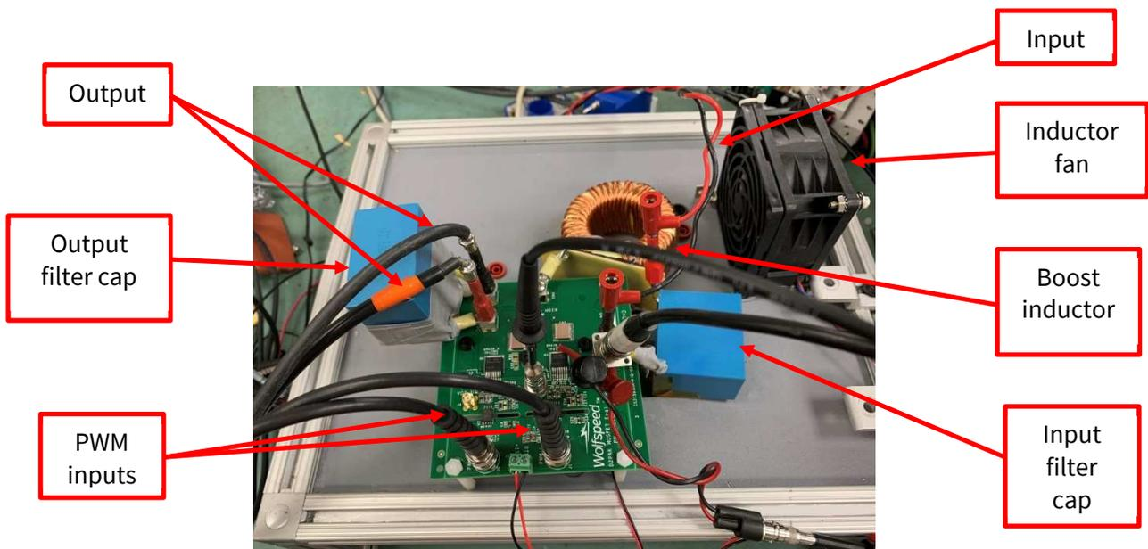
Figure 21: Synchronous boost converter setup
