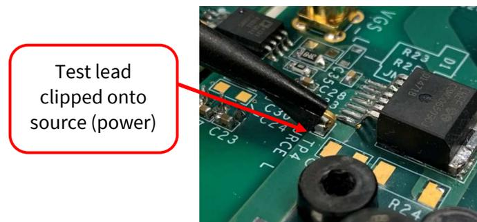
Figure 15: Test lead clipped on the source (power)
