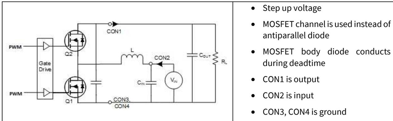
Figure 4: Synchronous boost converter configuration
