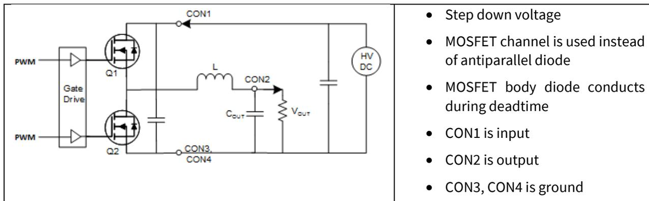
Figure 3: Synchronous buck converter configuration
