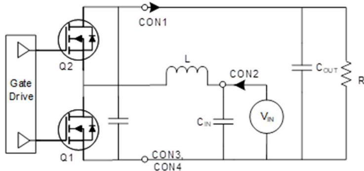
Figure 19: Synchronous boost converter schematic
