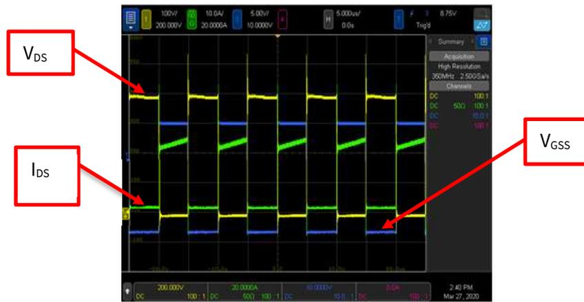
Figure 22: Switching waveforms of boost converter
