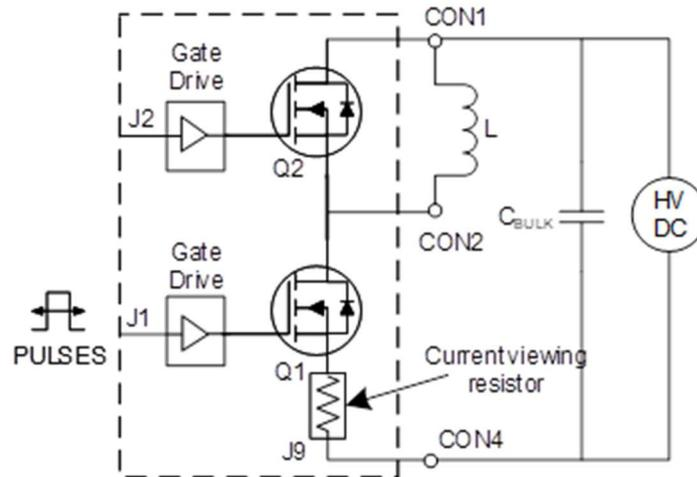
Figure 25: Clamped inductive switching measurement circuit
