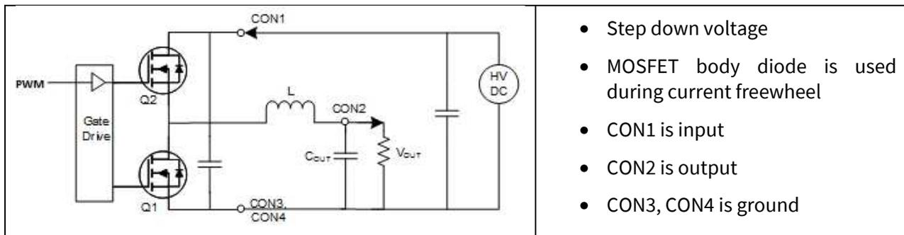
Figure 5: Asynchronous buck converter configuration
