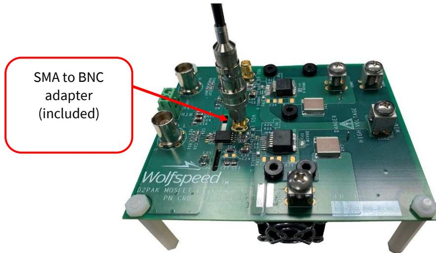
Figure 16: SMA to BNC adapter and X10 passive probe
