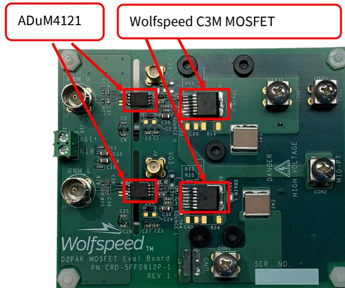
Figure 11: Gate driver and MOSFET locations
