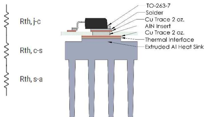
Figure 18: Thermal management stack up
