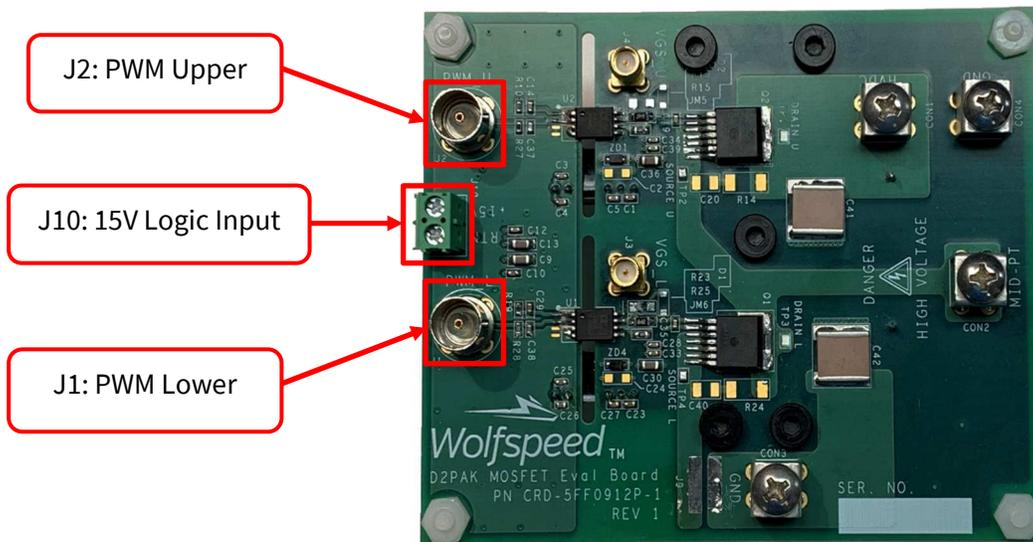
Figure 14: Low-voltage input connectors
