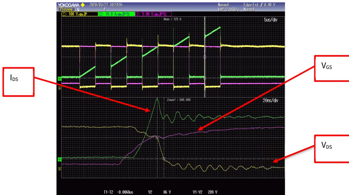
Figure 27: Double pulse waveform
