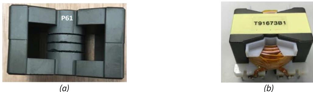
Figure 6: Low-profile transformer (PQ50/28 with material P61 from acme) with leakage inductance used for resonant inductor: (a) Magnetic core with distributed airgaps; (b) Experimental transformer prototype
